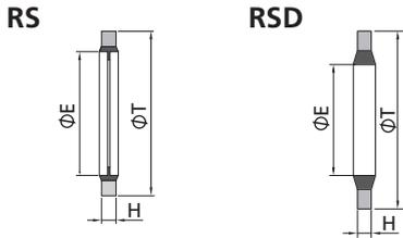
The RS and RSD gaskets provide a seal with male ISO parallel threads. The gasket consists of a fluorocarbon FKM or Buna inner ring bonded to a carbon steel or stainless steel outer ring.
