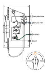
Turn the handle to the "PROCESS" position, allowing the sample to flow continuously into and fill the cylinder. Hold for a period of time to ensure representative sampling.
