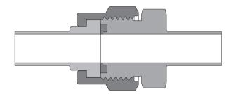
2. Tighten the nut 1/8 turn with a wrench while holding the fitting body steady.
